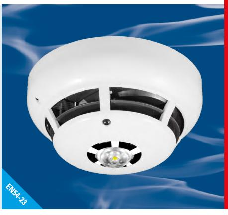
The Protec Algo-Tec™ 6000*PLUS* sensor range have been developed to incorporate advanced fire sensing technology, electronic sounders, high intensity LED visual alarm devices (VAD) and speech enhanced talking sounder capability, all integrated within the sensor head and powered from the loop.
